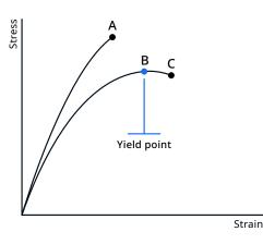
A. Tensile stress at break, elongation at break (no yield point) B. Tensile stress at yield, elongation at yield
