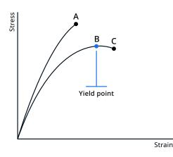
A. Tensile stress at break, elongation at break (no yield point) B. Tensile stress at yield, elongation at yield
